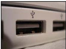
The **Universal Serial Bus** is a multipurpose port. USB connects devices such as jump drives, printers, digital cameras, etc.
